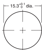
Panel Cutout Dimension Panel thickness = 1 to 4 mm
